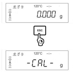
⇒ Wait until the weighed value for the required adjustment weight appears flashing.
