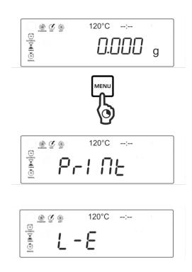
Acknowledge with The protocol of the measurement carried out as last is displayed under the ident number "1". The instrument stores the last five protocols (ident number 1 -5). With every new measurement, the ident number One will be overwritten.
